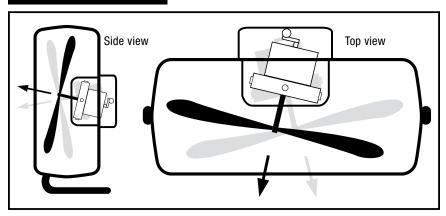
The rotor of the fan blade oscillates a full 360° allowing for maximum coverage in your space.
