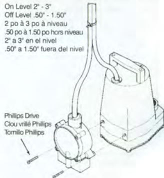
Figure 1 RS-5LL Mounted to 5-MSP RS-5LL fixé à 5-MSP RS-5LL montado a la 5-MSP
